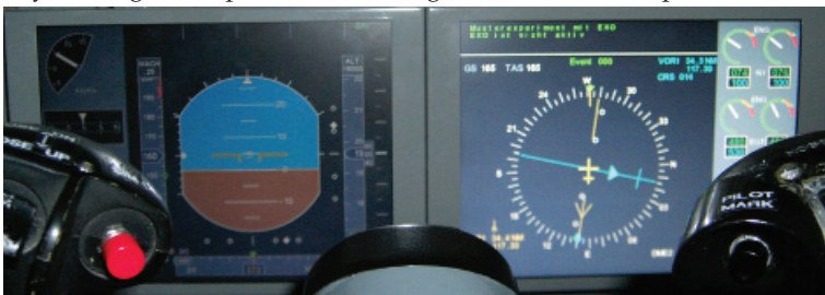
Fig. 2. Typical primary flight display and navigation display
