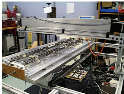
Fig. 51. Morphing wing system in the bench test
